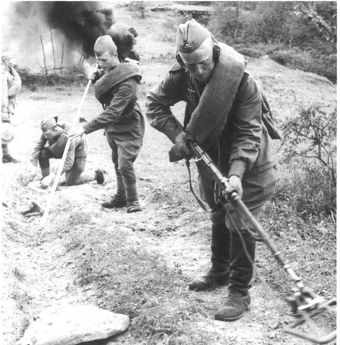
Right Mine clearing on a Rumanian mountain road. Red Army sappers' tasks were fully recognized as dangerous. As Soviet soldiers grimly put it, "our sappers never make more than one mistake". This mine-detecting system cleverly attaches the detector to the rifle barrel, placing greater distance between the sapper and any mine. The senior soldier with the detector evidently has a gallantry award.
