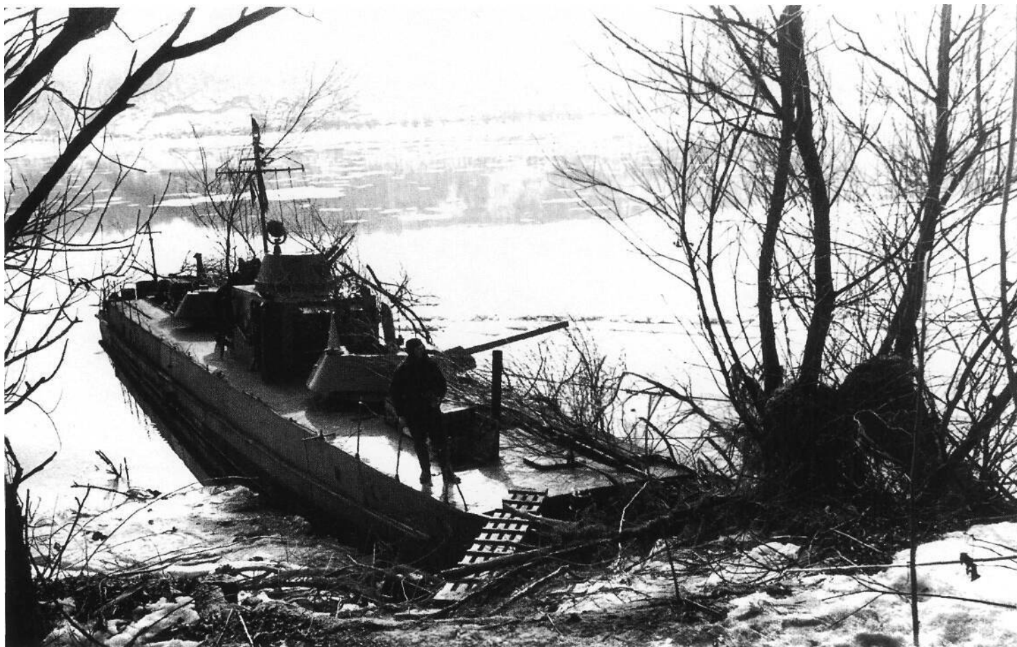
Above A gunboat of the Danube Flotilla, commanded by Rear Admiral Georgii Kholostyakov. These gunboats provided fire support to Soviet infantry in the assault on Budapest. They also transported troops, ammunition and supplies and carried out mine-sweeping. Their fire-power was supplied by bolting a tank turret to the deck.
